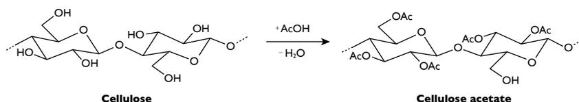
Cellulose, acetic acid, and acetic anhydride are mixed together and reacted to form cellulose acetate polymers. This process is aided by the addition of a small amount of sulfuric acid which is subsequently neutralized during processing.
